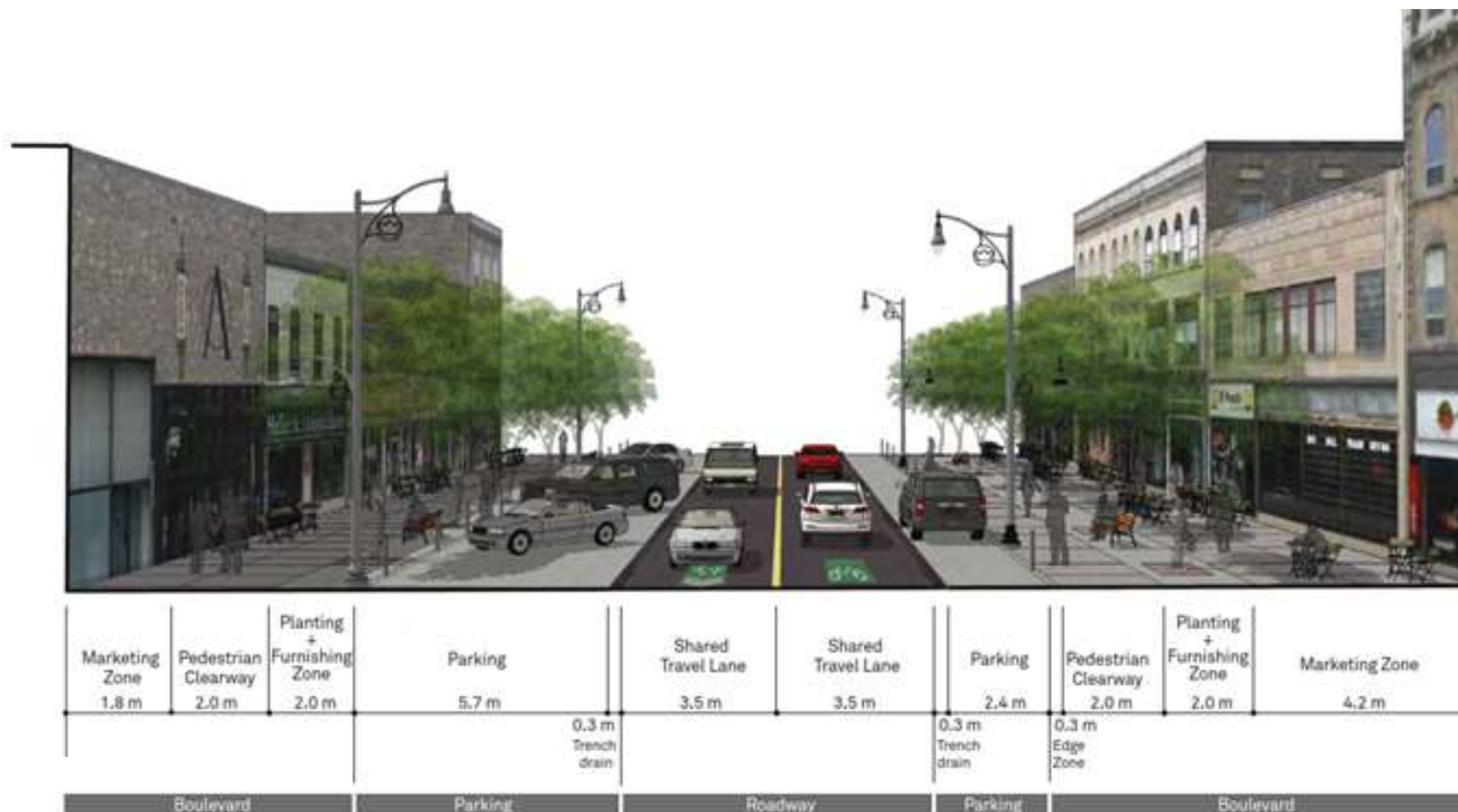
4a) Two-lane Configuration with Shared Use Lanes and Angled Parking on One Side of Street
