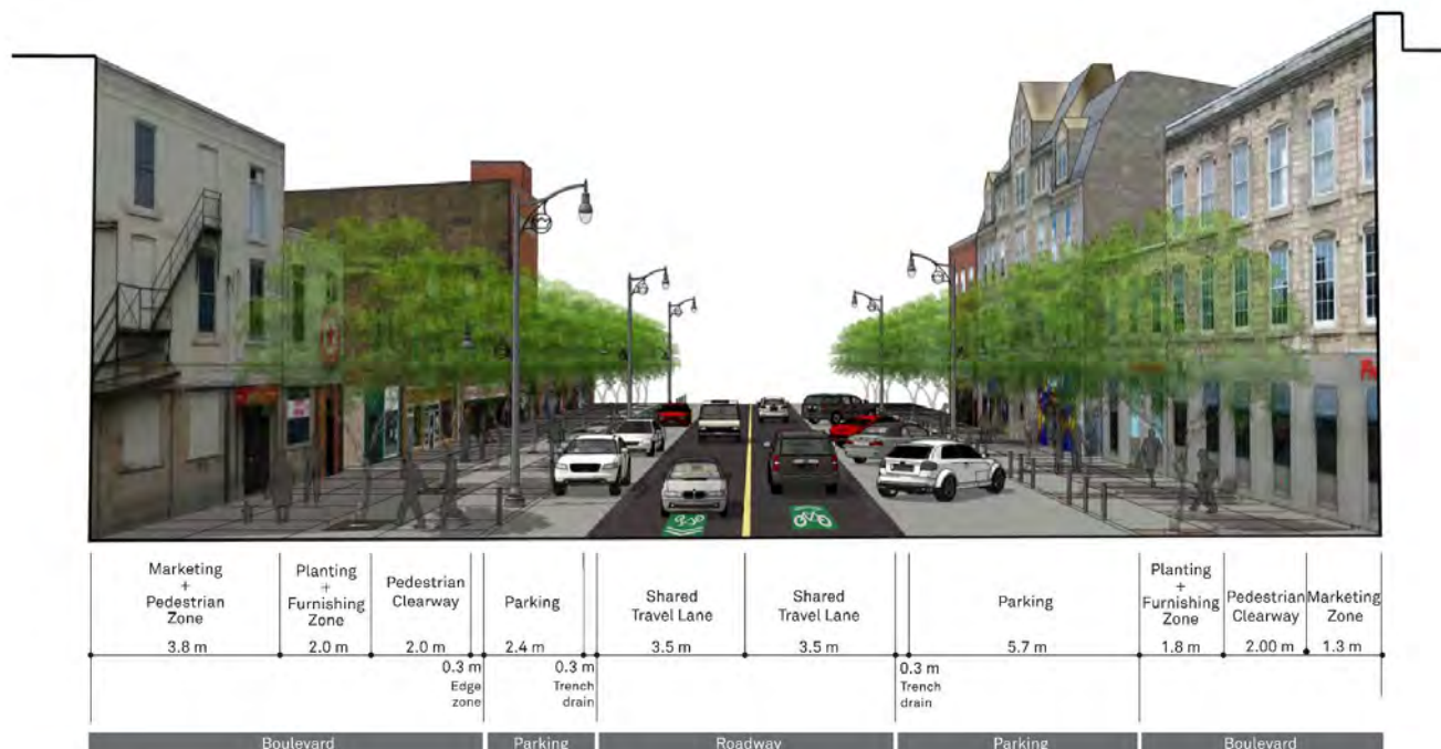
4a) Two-lane Configuration with Shared Use Lanes and Angled Parking on One Side of Street
