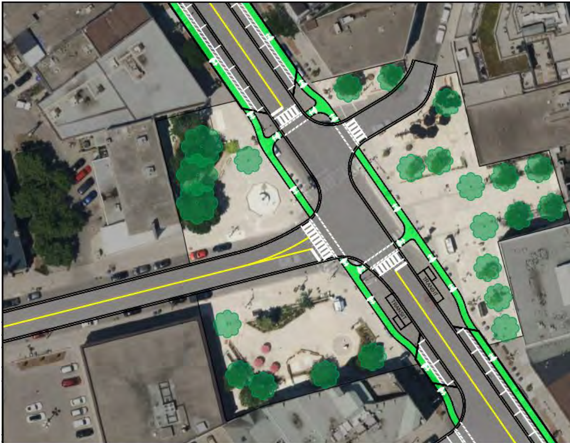
Figure 6-3: Recommended Intersection Configuration
