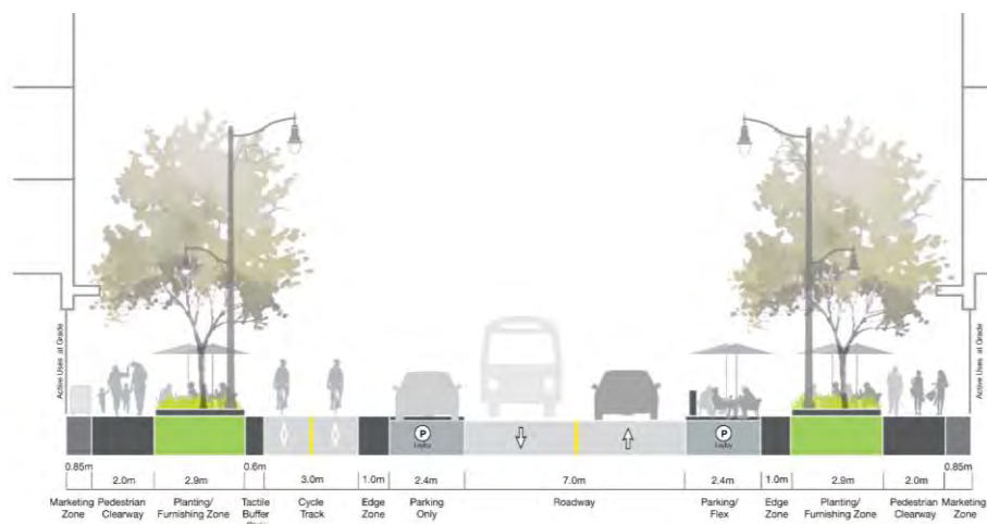
Exhibit 3-7: 2-Lane Configuration with Bi-Directional Cycle Track and Flex on One Side of Street
