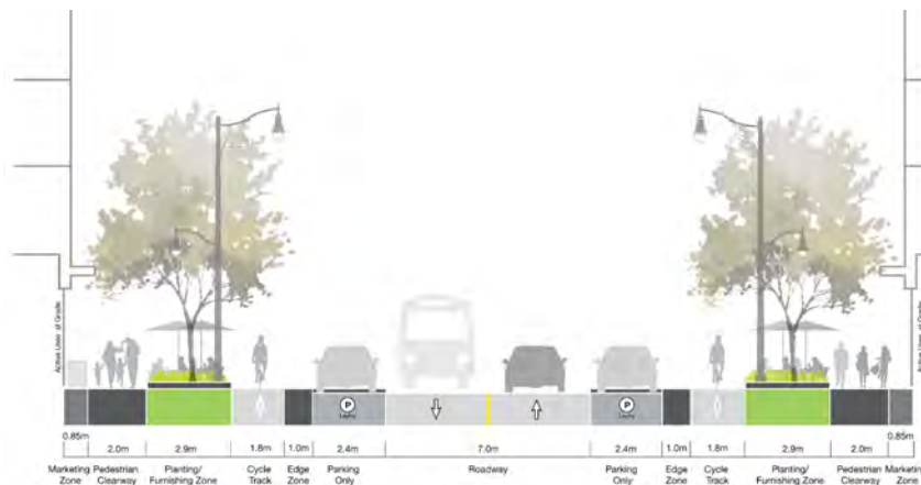
Exhibit 3-5: 2-Lane Configuration with Uni-Directional Cycle Track and Flex on One Side of Street
