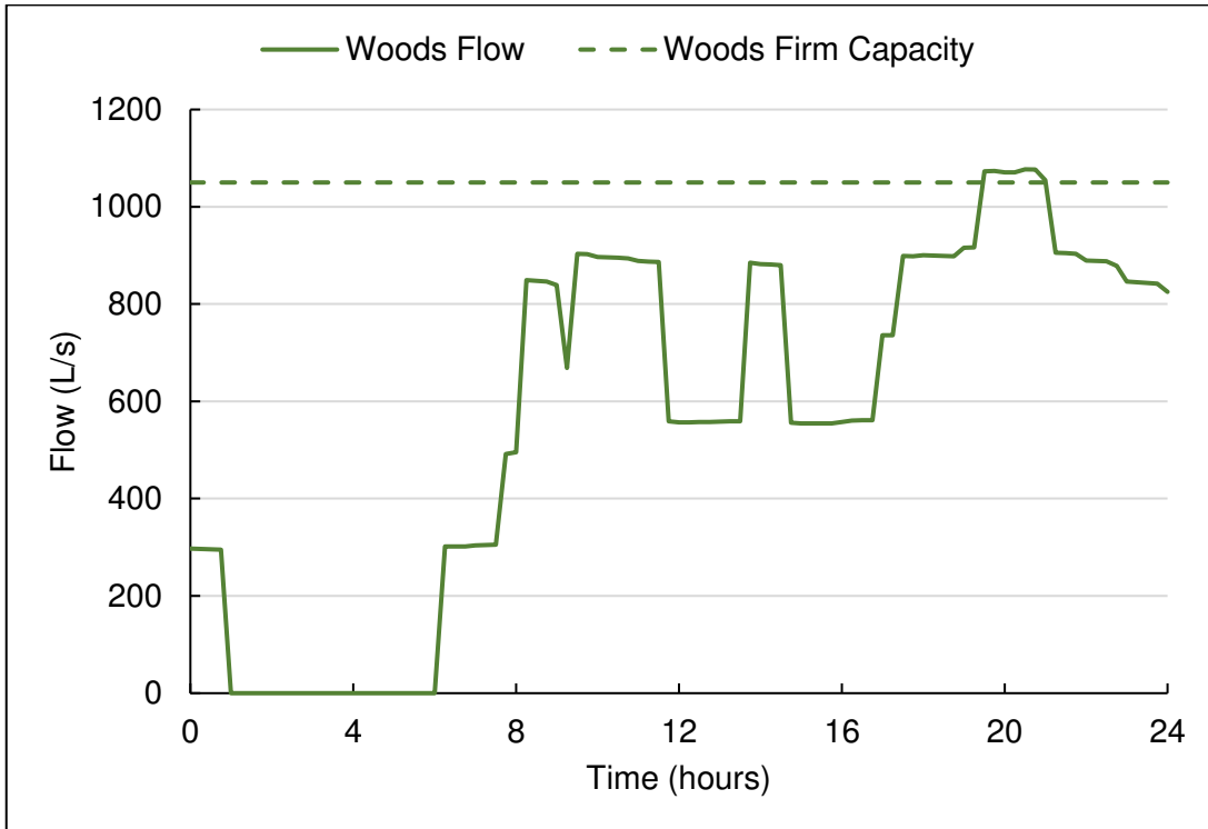
Figure 3-23 2051+ MDD – Woods Pump Station Flow
