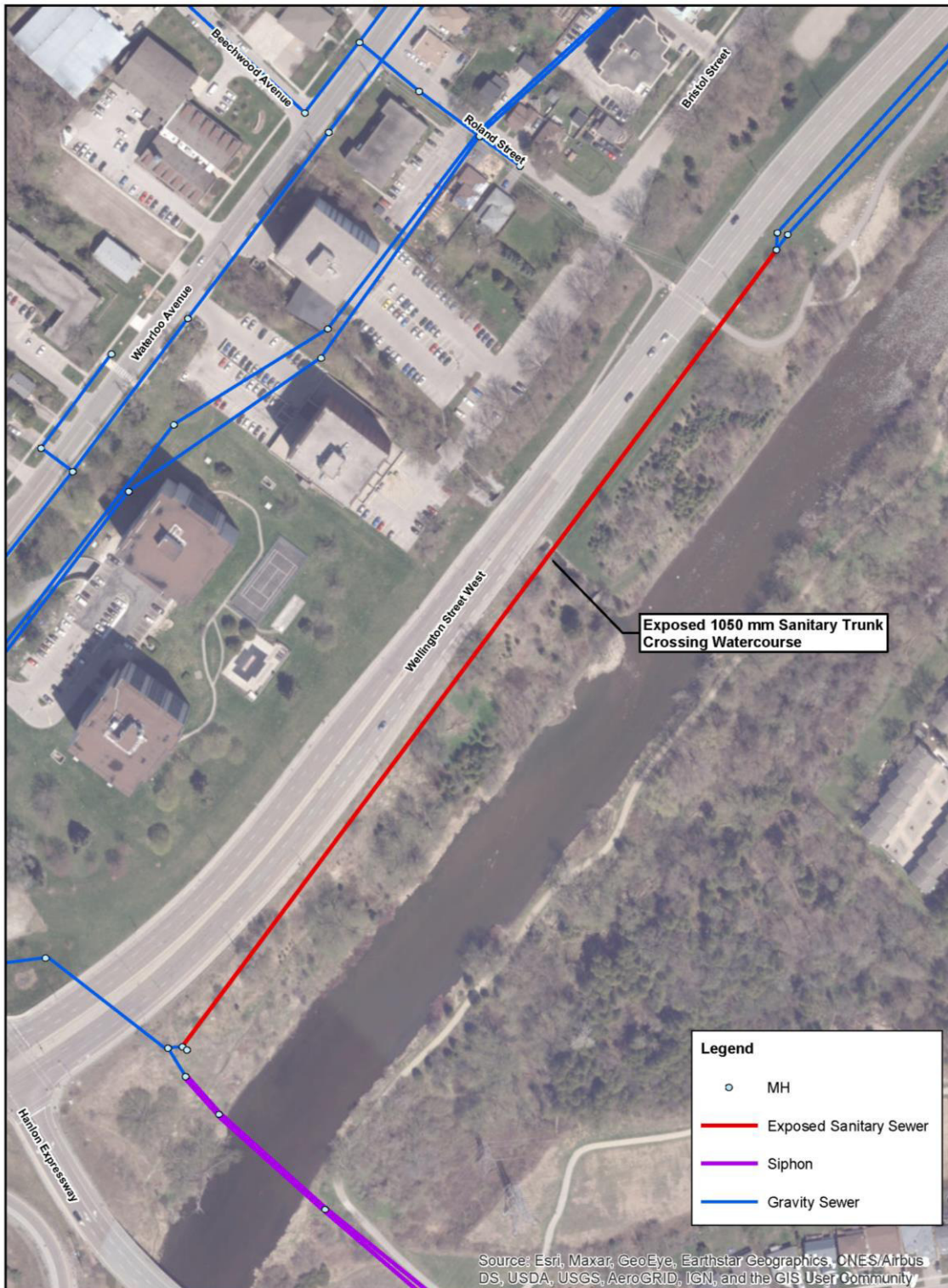
Figure 5-38 Exposed Sanitary Trunk
