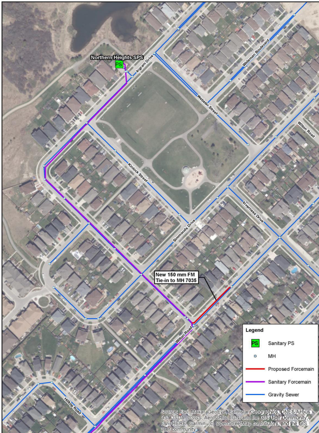
Figure 5-16 Northern Heights PS Diversion Concept
