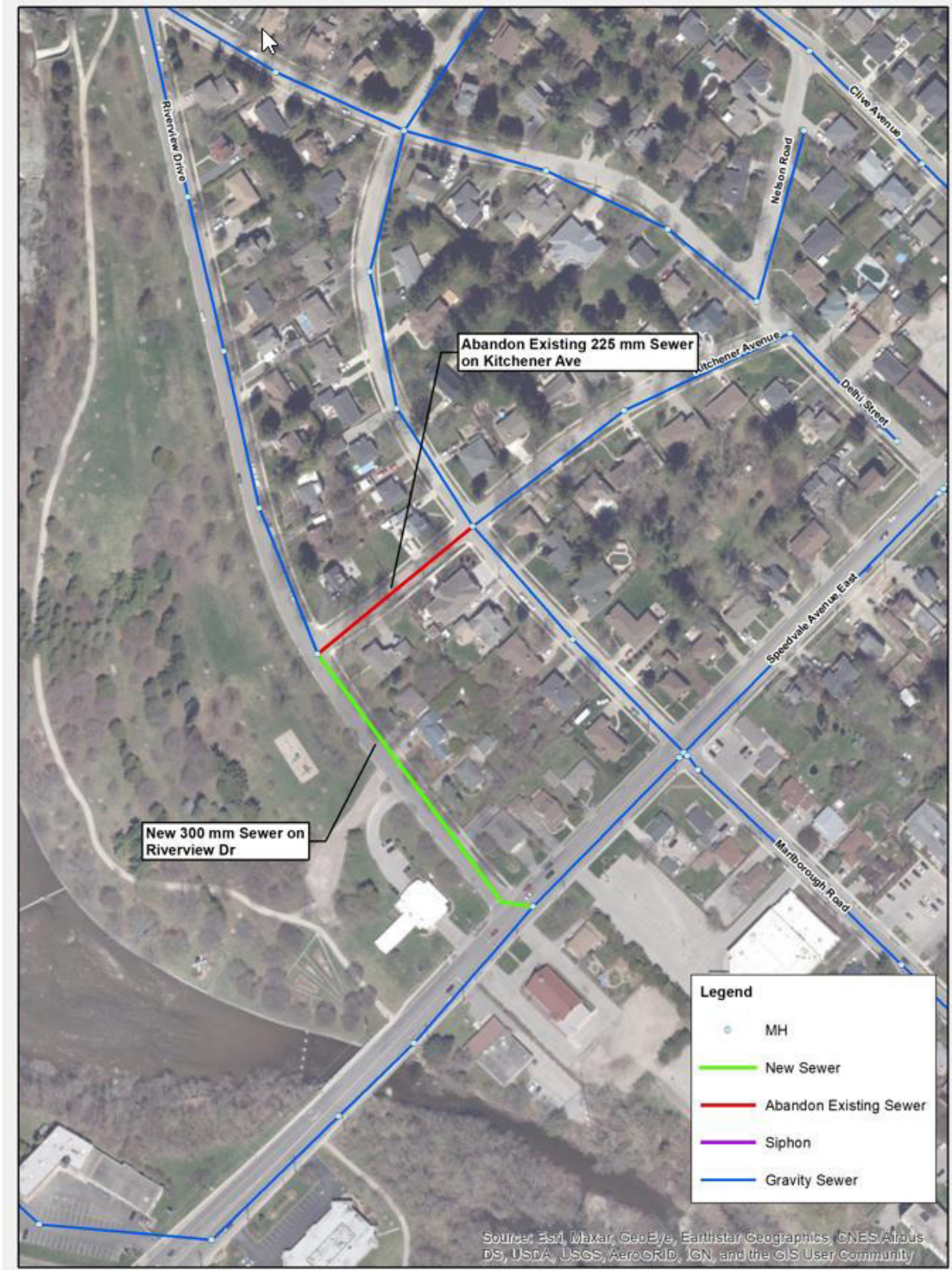
Figure 5-17 Reach 2-3 Sewer Realignment
