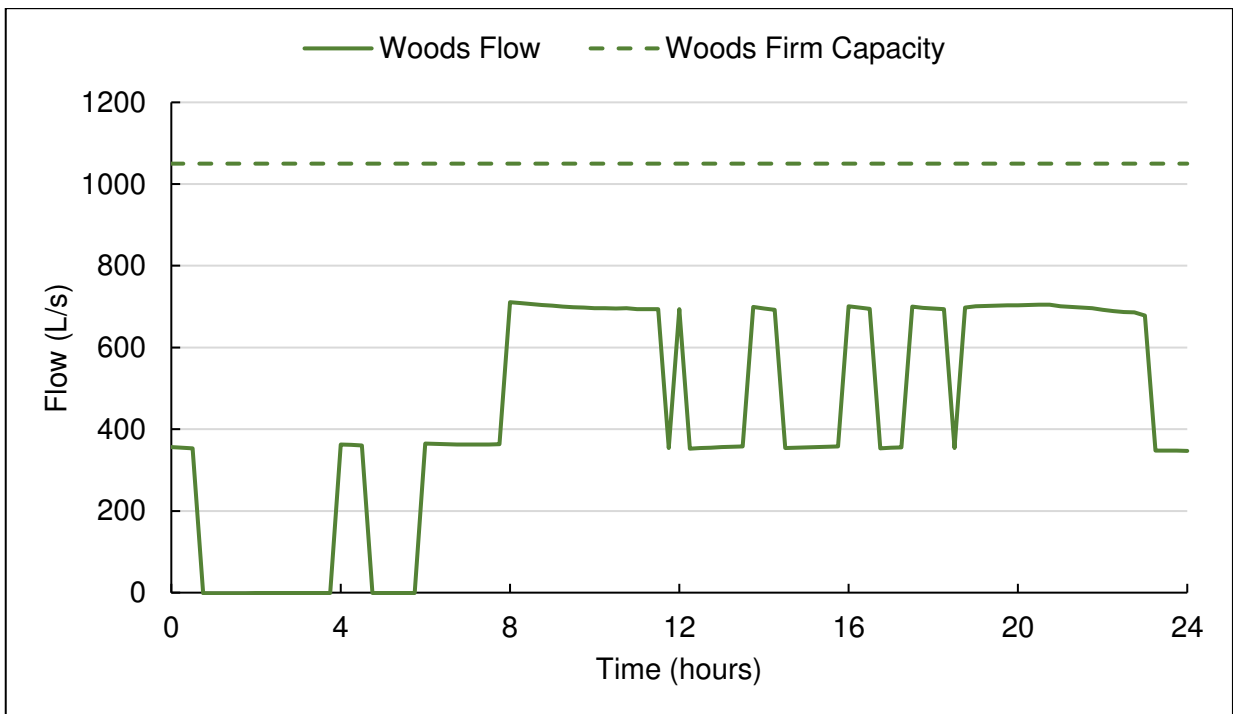
Figure C-2031-14 2031 MDD PS Flows – Proposed Upgrades Active – Arkell PS Off
