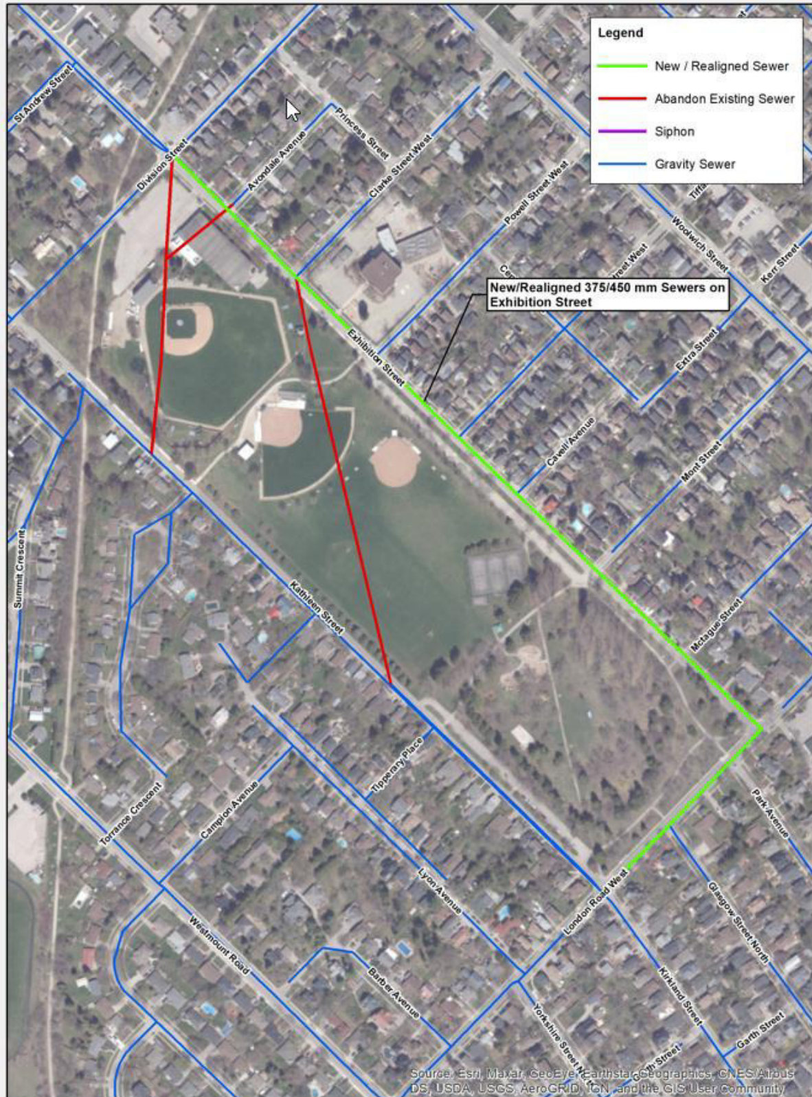
Figure 5-22 Reach 3-1 Sewer Realignment
