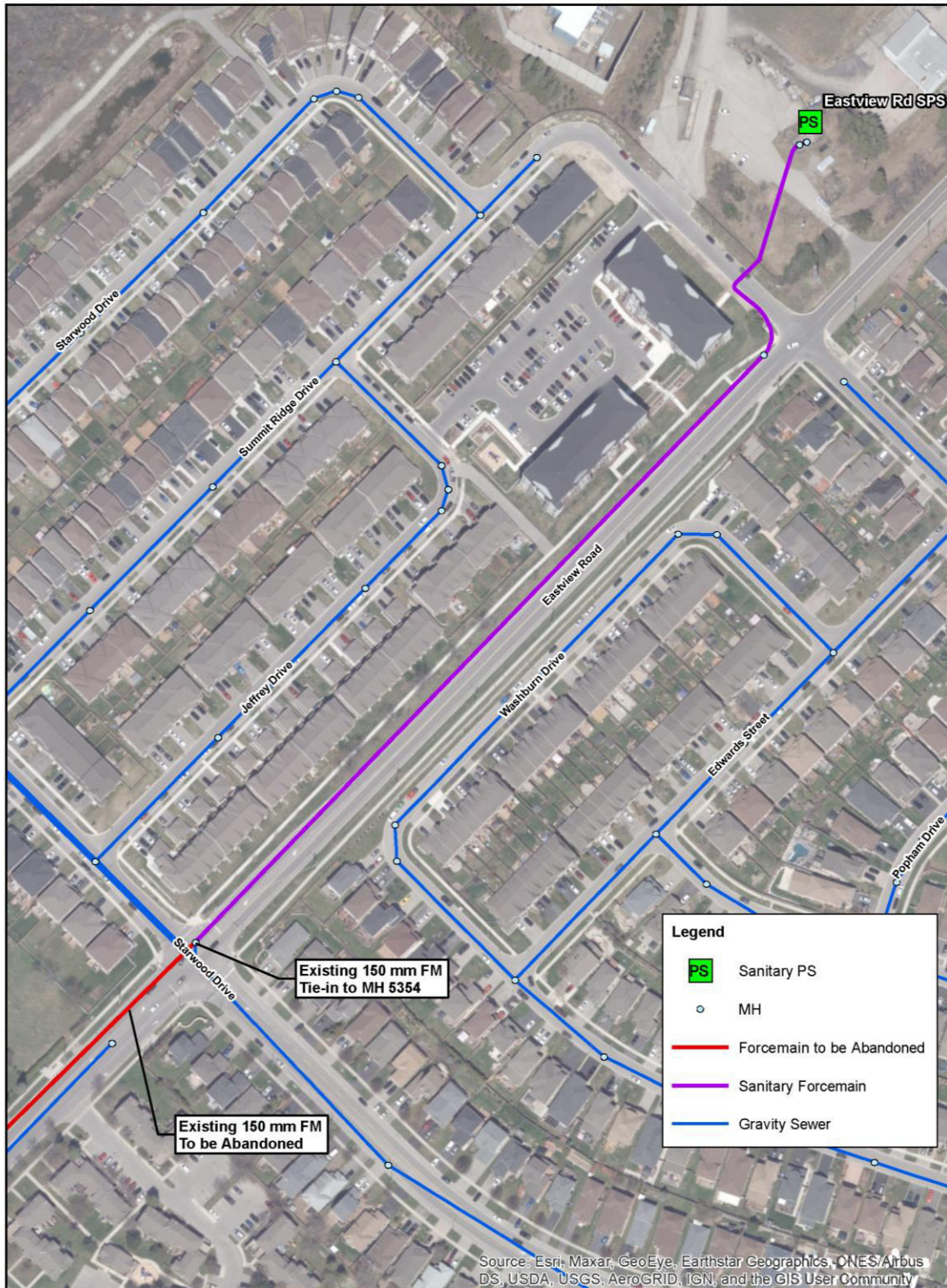
Figure 5-25 Easview Road PS Diversion Concept
