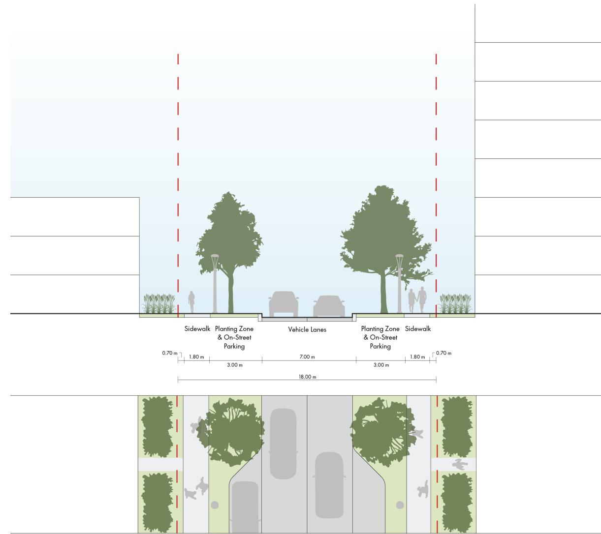
Figure 4.8 - Proposed Local Street cross section in accordance with Secondary Plan requirements and City of Guelphs Complete Street Guidelines
