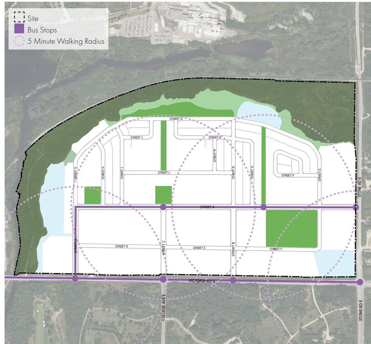
Figure 3.4 - Proposed transit network for the Draft Plan of Subdivision, including bus stop locations
