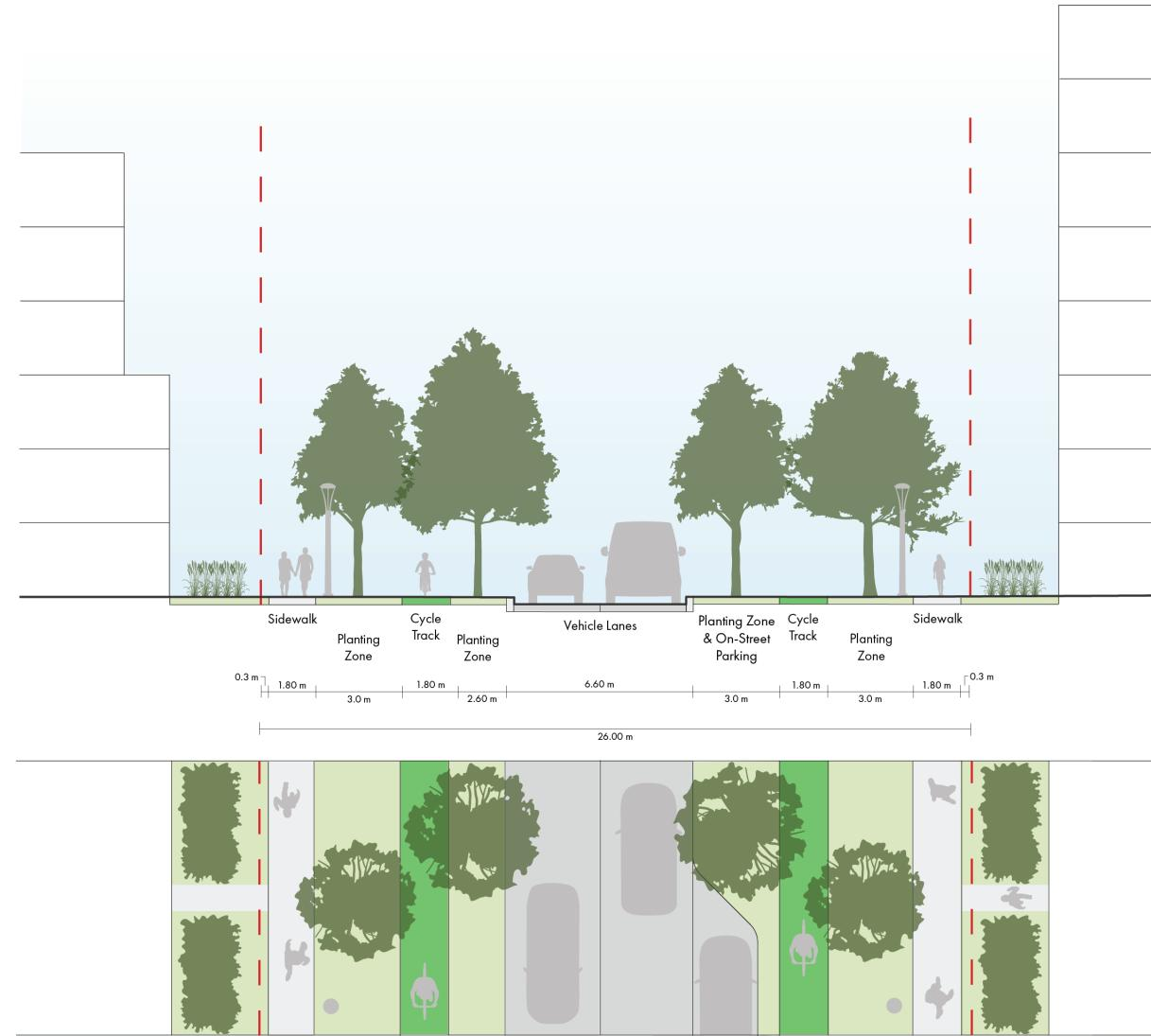
Figure 4.7 - Proposed Collector Street cross section in accordance with Secondary Plan requirements and City of Guelph's Complete Street Guidelines
