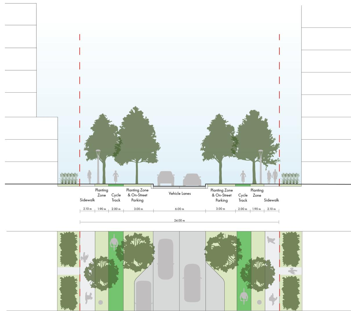
Figure 4.6 - Proposed Main Street cross section in accordance with Secondary Plan requirements and City of Guelph's Complete Street Guidelines
