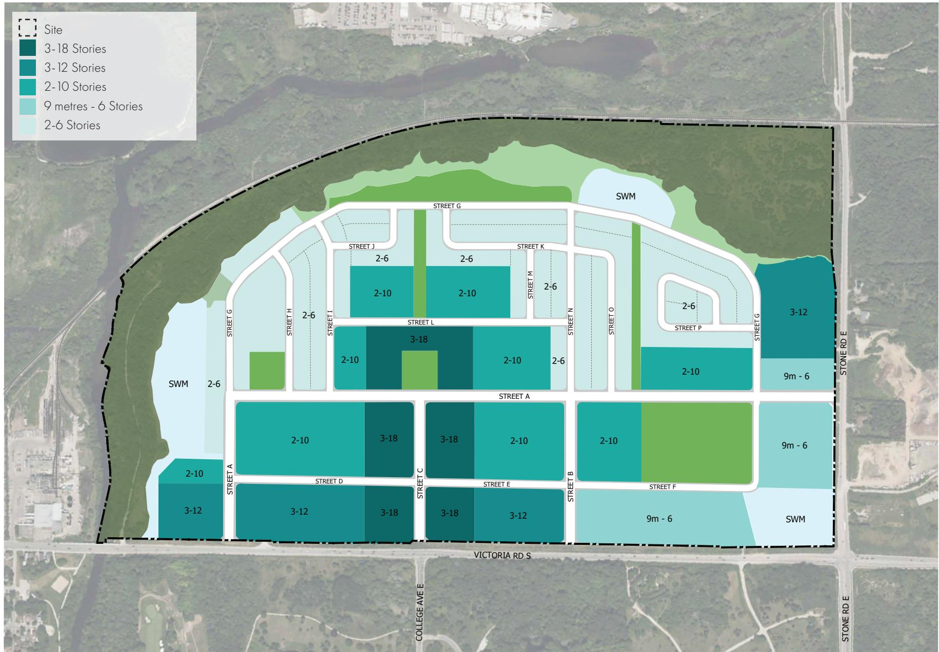
Figure 3.2 - Proposed building height hierarchy, showing the tallest buildings in the mixed-use district, with building heights transitioning down towards the edge of the abutting natural heritage lands
