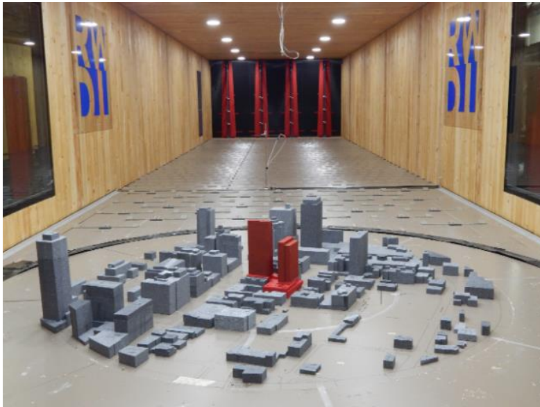
Figure 3b: Photo of Modelled Buildings in a Boundary-layer Wind Tunnel
