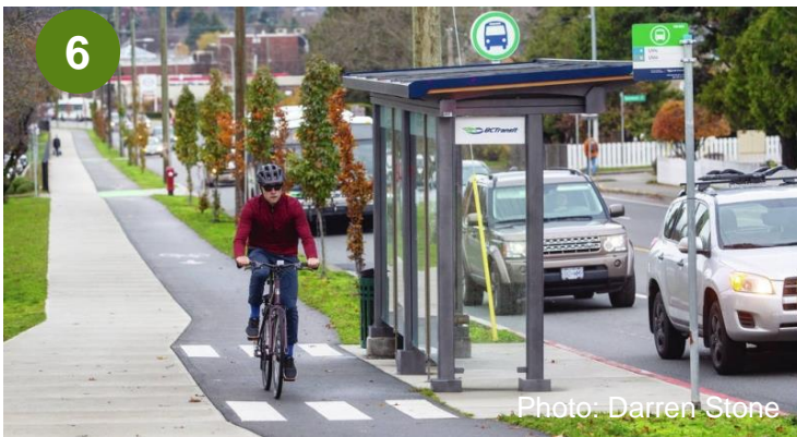
Example of transit stop with cycle track.
