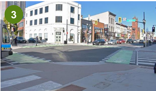
Example of protected intersection.
