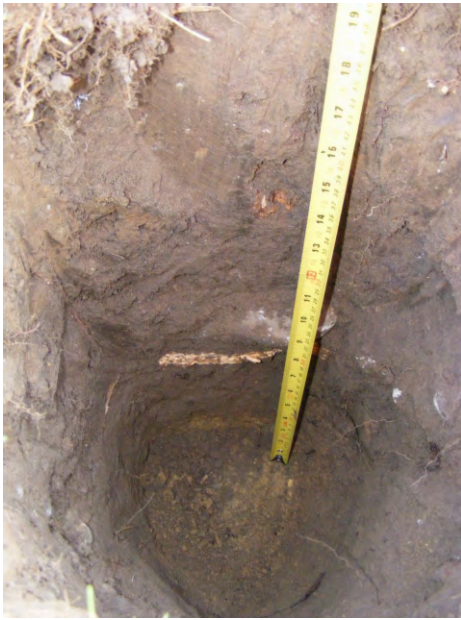
Plate 13: Test pit showing fill in former ditch beside driveway, looking NW (Photo 7296).
