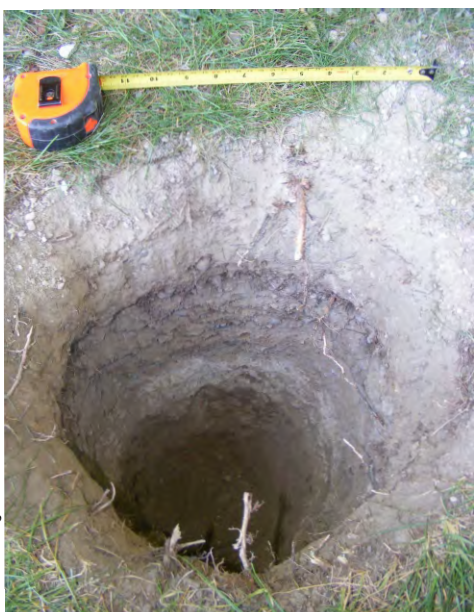
Plate 11: Test pit showing layers of fill in disturbed area beside driveway, looking W (Photo 7282).
