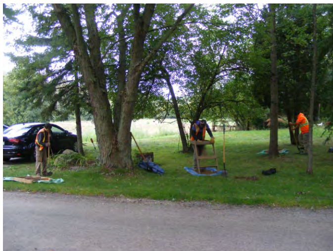
Plate 10: Crew test pitting in an area of fill north of the former pond, looking W (Photo 7346).
