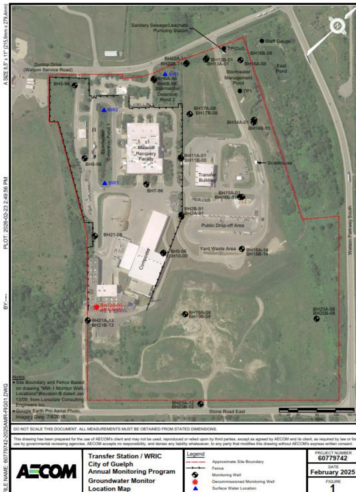
Figure 1: Groundwater Monitor Location Map
