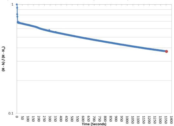
Time Lag:1356 secondsHydraulic Conductivity (m/s):2.6 x 10-7Soil Type:Silty fine sand to silt with some fine sand and clayNotes:Slug in, falling head
