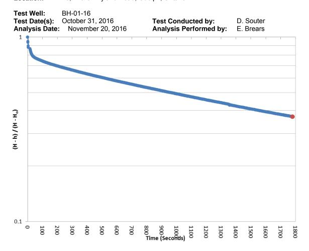
Time Lag:1779 secondsHydraulic Conductivity (m/s): $3.2 \times 10^{-7}$ Soil Type:Fine silty sandNotes:Slug out, rising head
