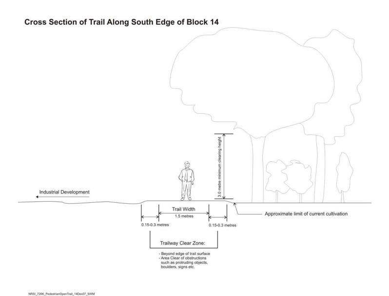
Figure 11. Pedestrian and Off-Road Trail Along South Edge of Block 14
