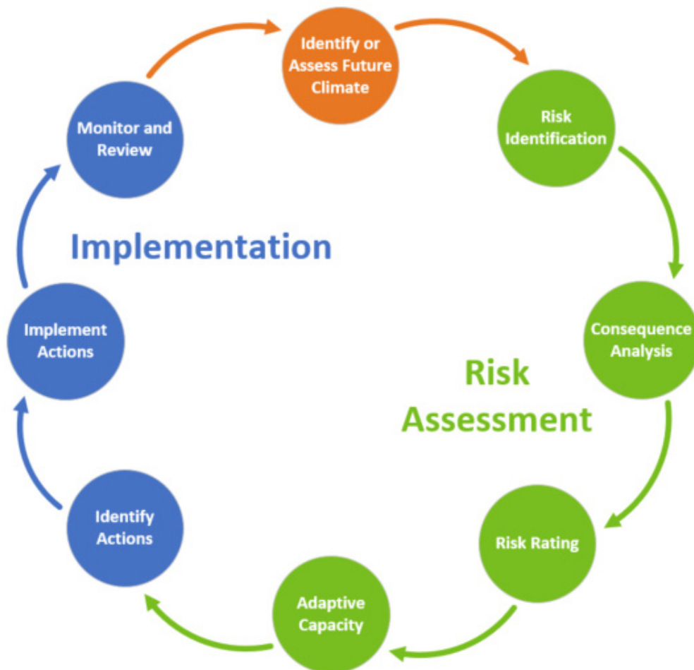
Figure ES.4 Risk Assessment, Implementation, and Monitoring Steps (Source: adapted from ISO 31000)
