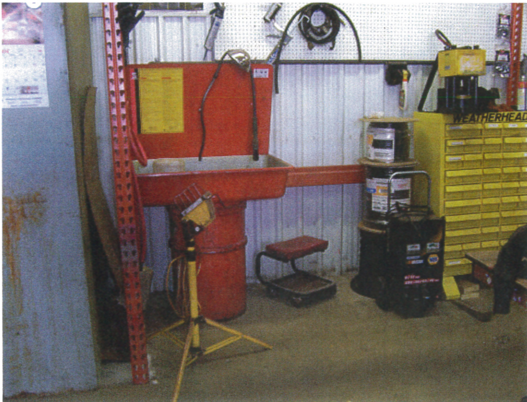
Photograph 2: A view of the parts cleaner in the workshop.
