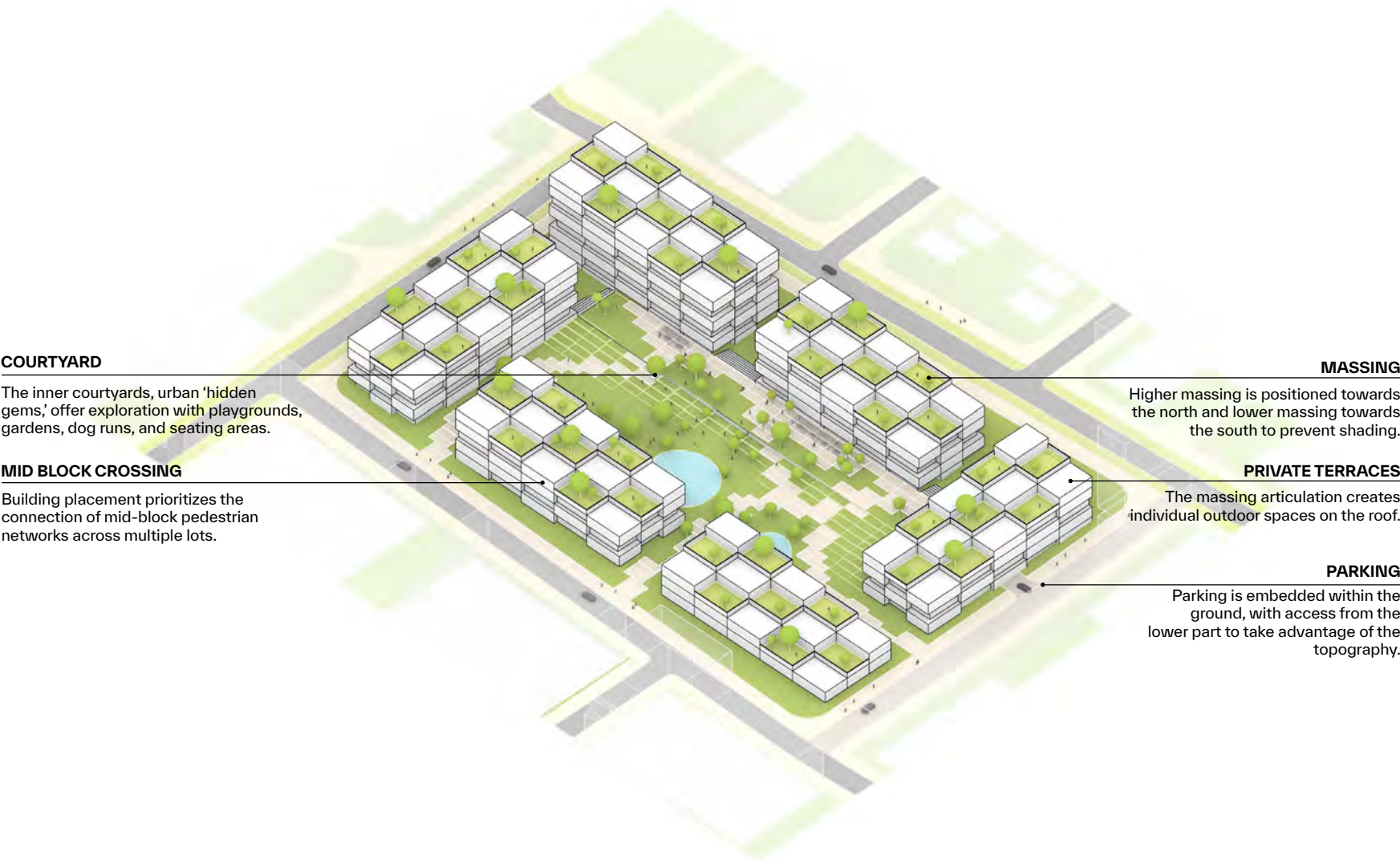
FIGURE: Diagrammatic example of development within a High-Density Mixed-Use district. Green roof placements are for illustrative purposes.
