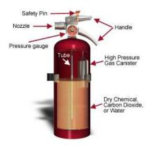
The proper type of extinguisher shall be used depending on the class of fire:
