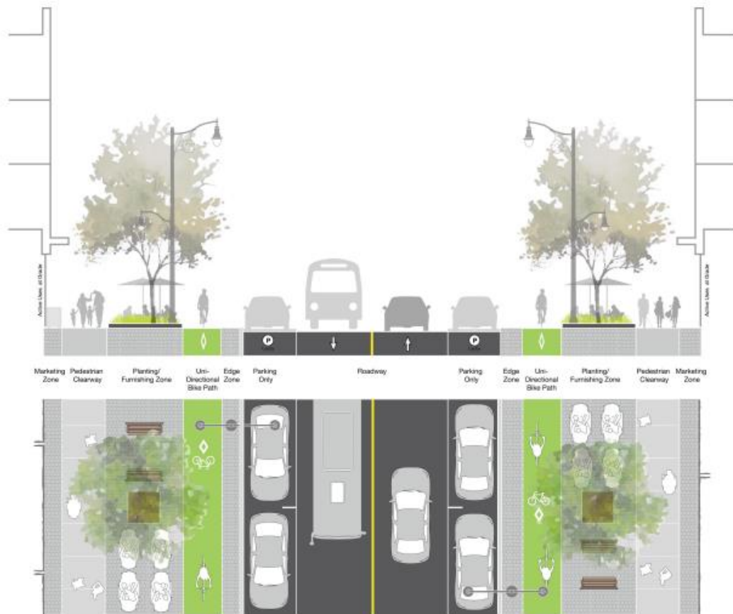
Figure 2: Recommended Wyndham Street corridor design - two lanes with a uni-directional bike path
