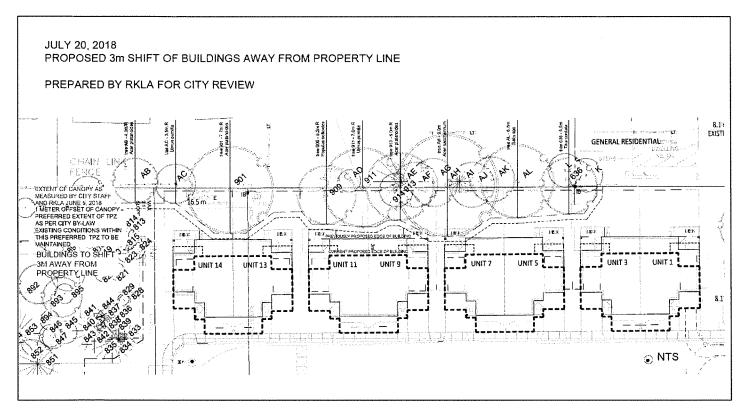
The TIPP clearly illustrates TPZs, the location of tree protection fencing, proposed site access and stockpile locations. Tree protection fencing is to follow City Standard SD-90a and SD-90c which can be found on the City's website under Part 'B' Contract Specifications 2016. The TIPP addresses trees that are in or within 10 m of the area of disturbance, including trees on neighboring properties.
