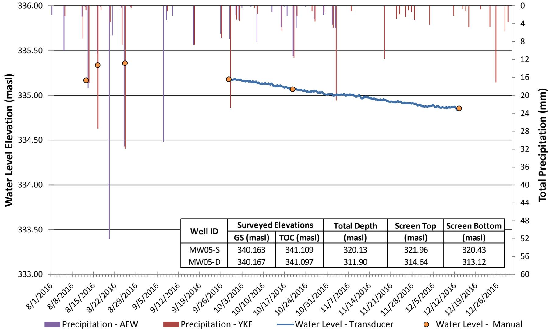
**Precipitation - AFW:** Data set from rain gauge installed by AMEC Foster-Wheeler at 500 Maltby Rd. E. **Precipitation - YKF:** Data set from weather station at Region of Waterloo International Airport (YKF).
