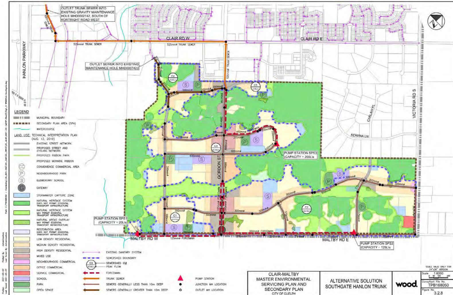
Figure EX.7. Preferred Wastewater Servicing Alternative
