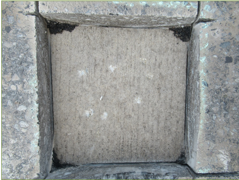
Photo S11 – Sawn Sample SS11 (light scaling)
