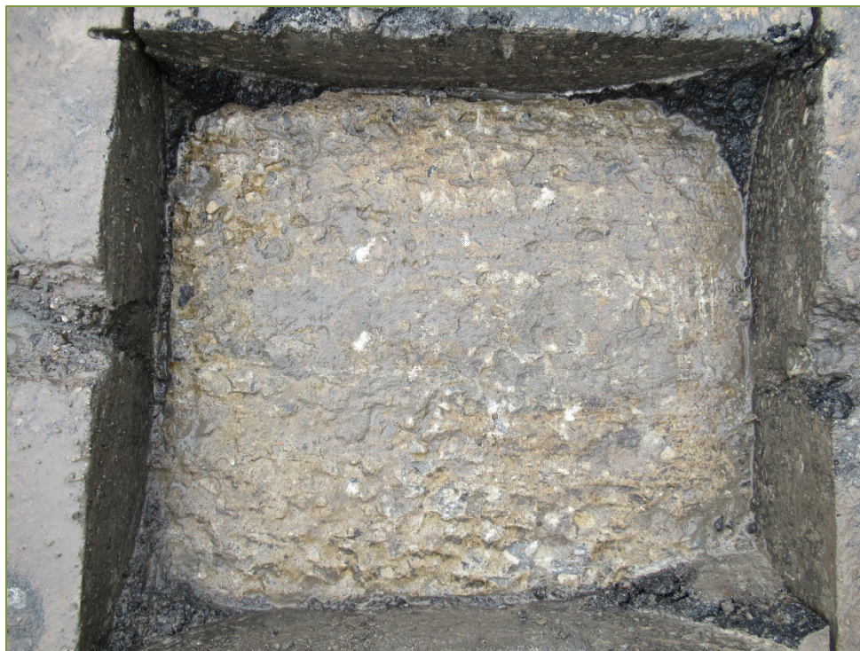
Photo S1 – Sawn Sample SS1 (medium scaling)
