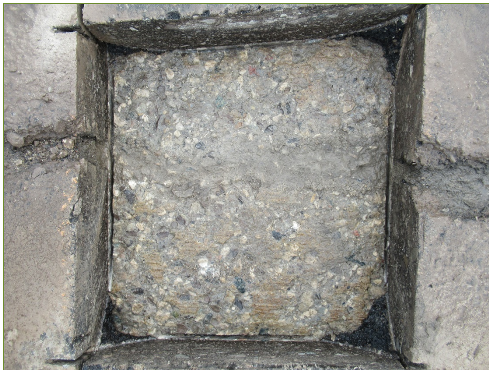
Photo S4 – Sawn Sample SS4 (medium scaling)
