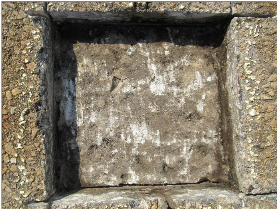
Photo S2 – Sawn Sample SS2 (rough surface)
