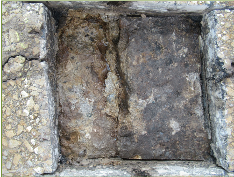
Photo S1 – Sawn Sample SS1 (crack, spall, and rough surface)
