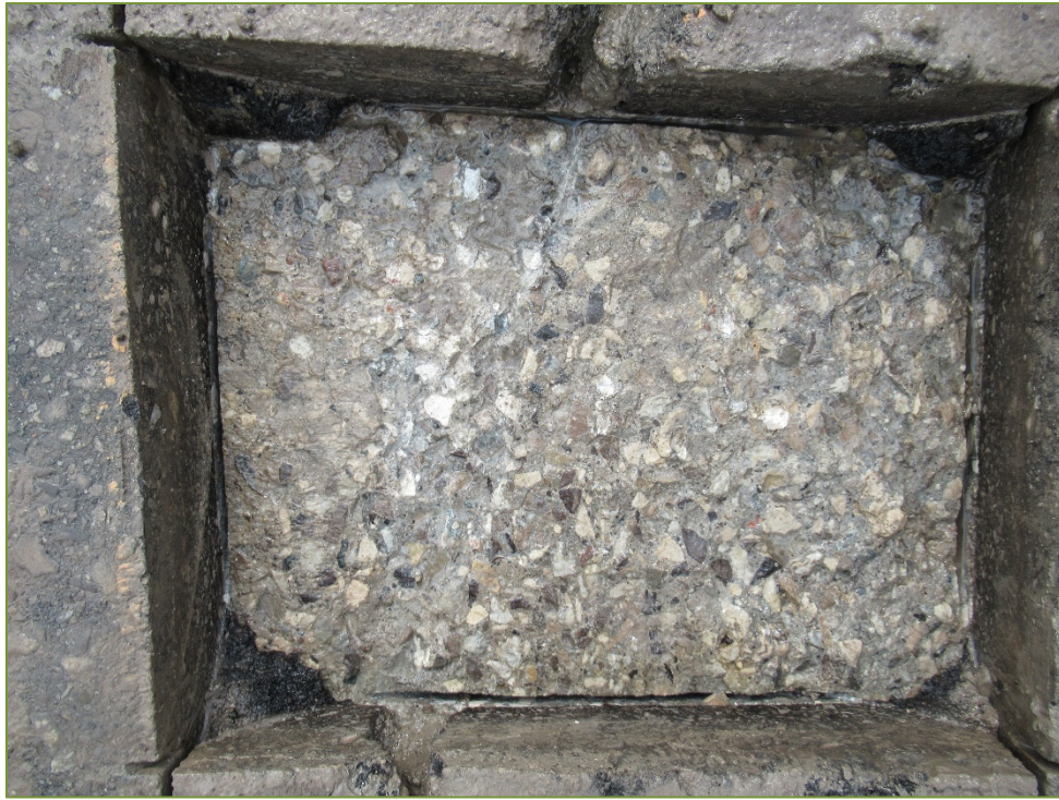
Photo S5 – Sawn Sample SS5 (severe scaling)
