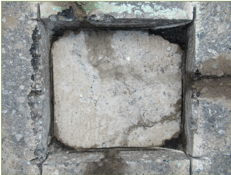
Photo S10 – Sawn Sample SS10 (crack, and medium scaling)
