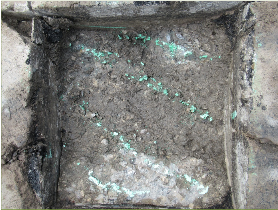
Photo S7 – Sawn Sample SS7 (delamination, and severe scaling)
