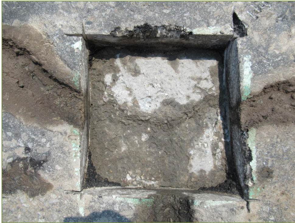
Photo S13 – Sawn Sample SS13 (severe scaling)
