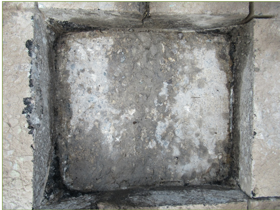
Photo S6 – Sawn Sample SS6 (medium scaling)
