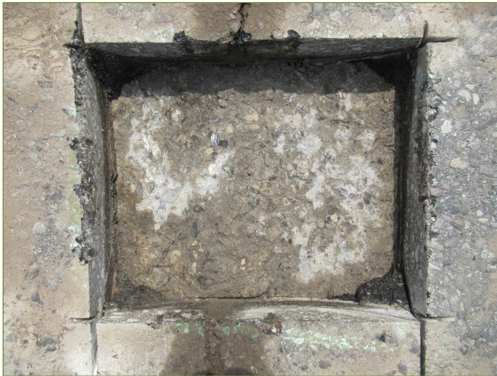
Photo S8 – Sawn Sample SS8 (medium scaling)
