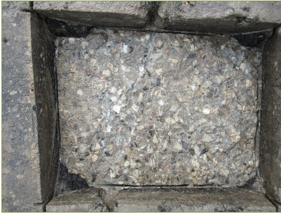
Photo S5 – Sawn Sample SS5 (severe scaling)
