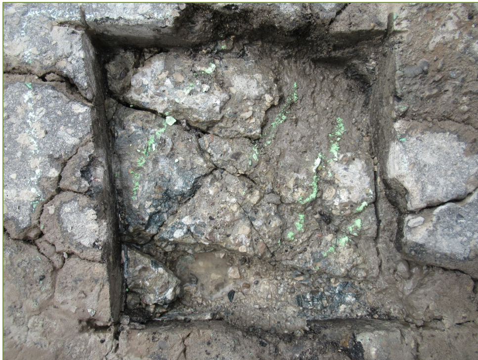
Photo S16 – Sawn Sample SS16 (cracks, delamination, and severe scaling)
