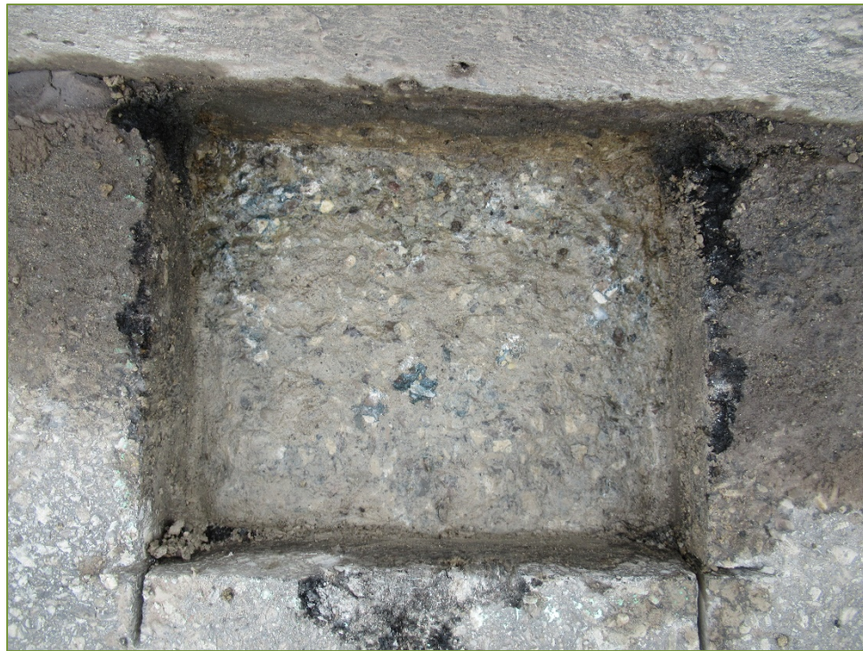
Photo S14 – Sawn Sample SS14 (severe scaling)
