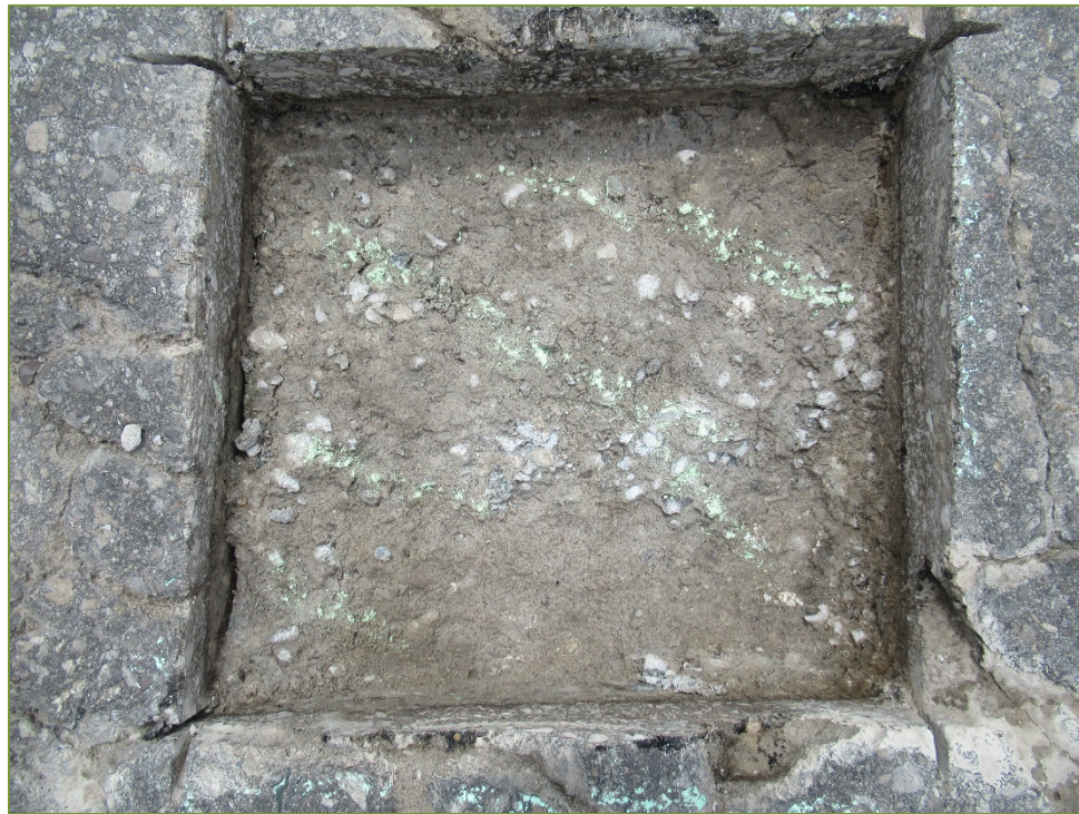
Photo S18 – Sawn Sample SS18 (delamination, and severe scaling)
