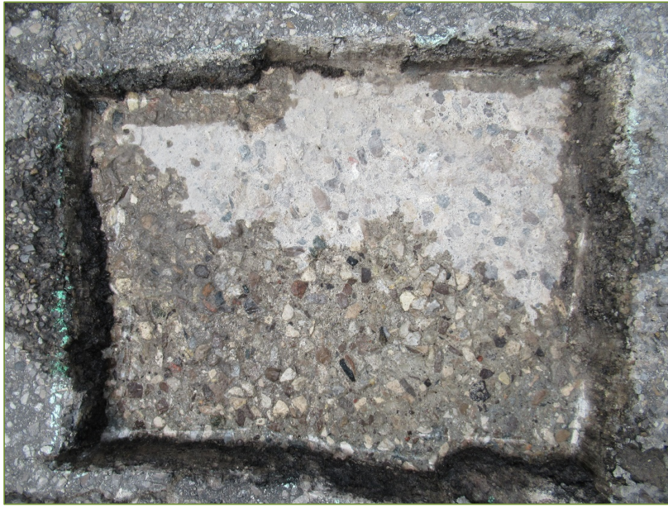
Photo S17 – Sawn Sample SS17 (medium scaling)
