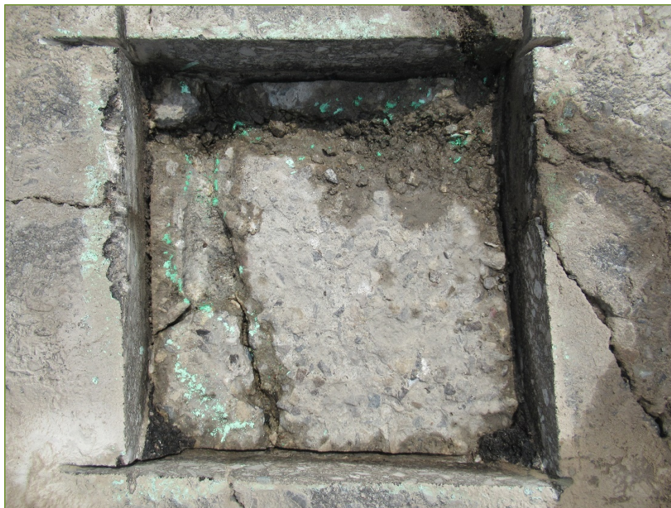
Photo S9 – Sawn Sample SS9 (delamination, and severe scaling)
