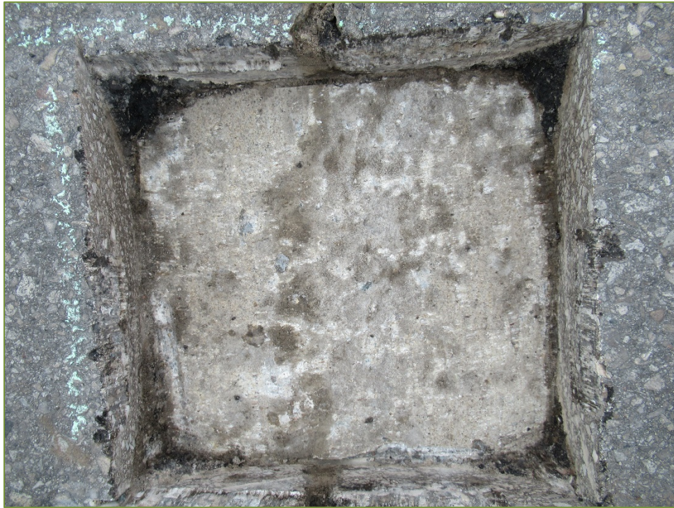
Photo S15 – Sawn Sample SS15 (light scaling)
