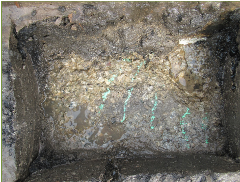
Photo S2 – Sawn Sample SS2 (delamination, and severe scaling)
