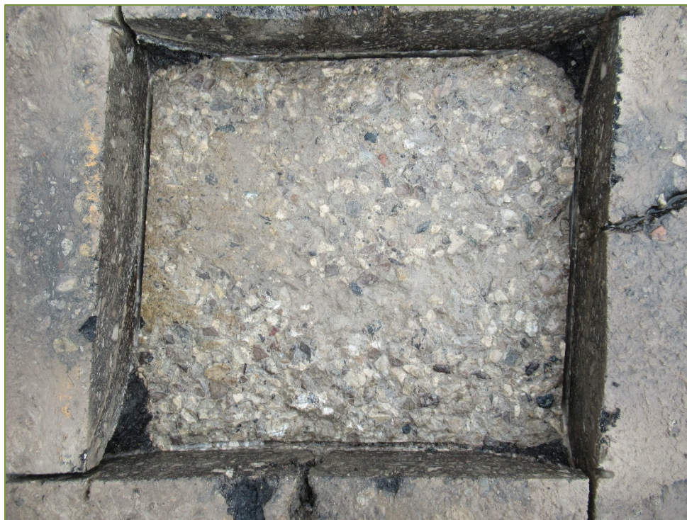
Photo S3 – Sawn Sample SS3 (medium scaling)
