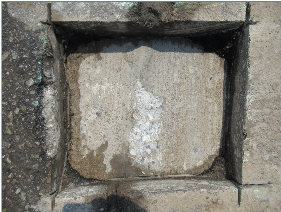
Photo S12 – Sawn Sample SS12 (light scaling)
