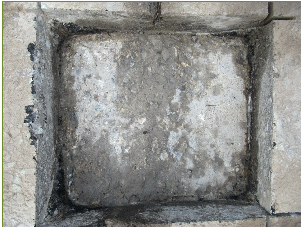
Photo S6 – Sawn Sample SS6 (medium scaling)
