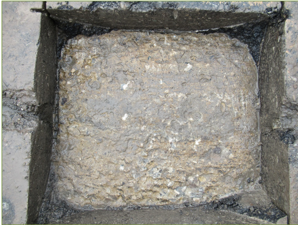
Photo S1 – Sawn Sample SS1 (medium scaling)
