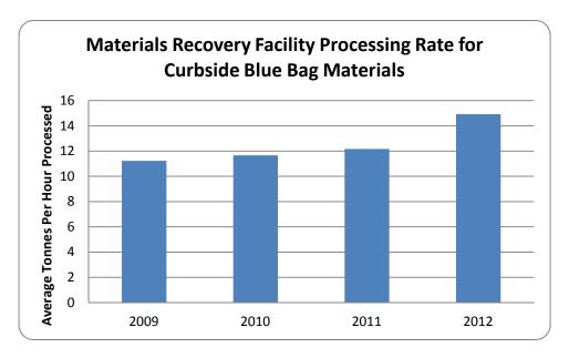
At the end of 2011 a drum feeder was installed in the Material Recovery Facility, replacing the old bag breaker. This change in equipment achieved a 23% increase in actual tonnes per hour processed of blue bag material (14.93 T/hr in 2012). Our new processing goal is 15 tonnes per hour compared to our previous goal of 12 tonnes per hour.
