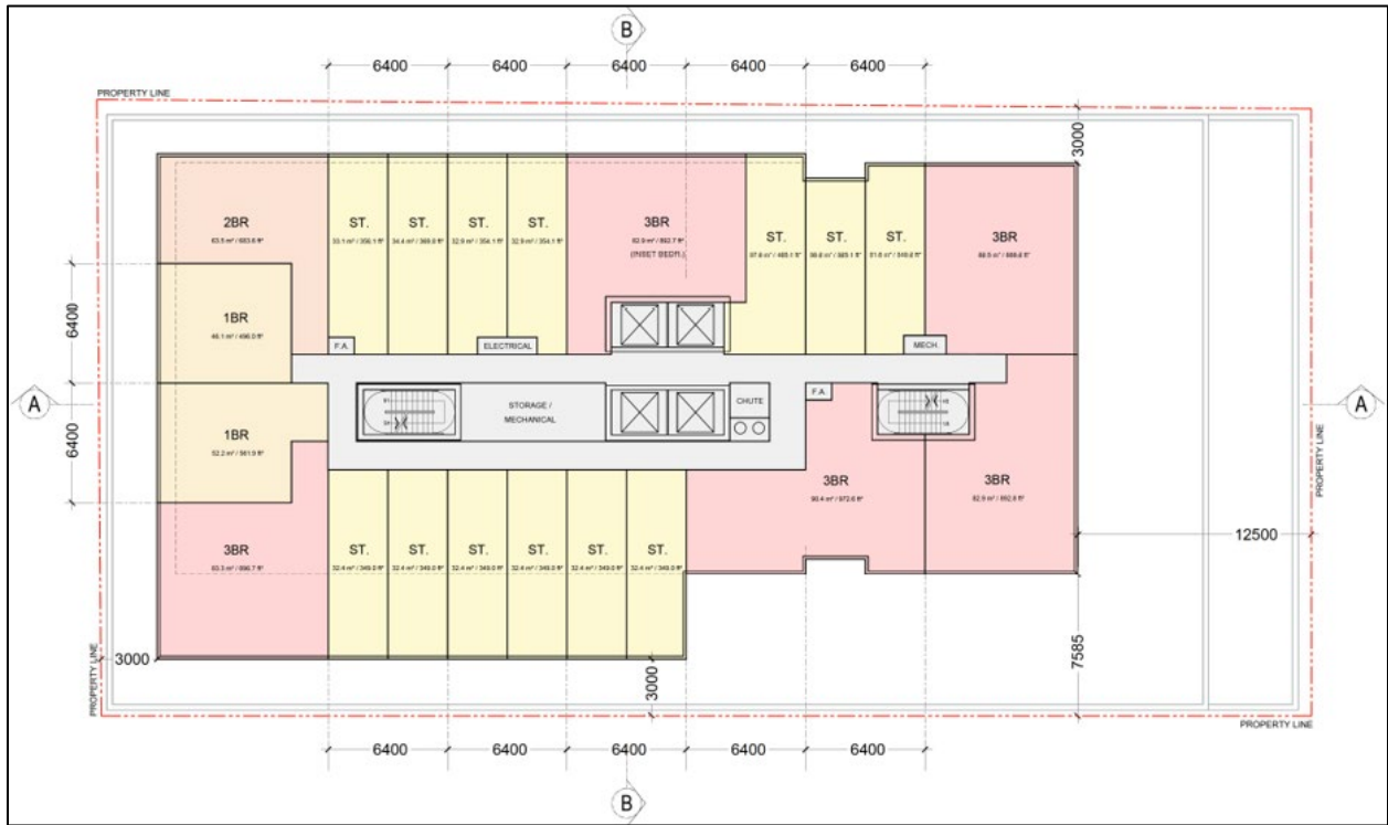
Figure 18: 6 th to 8 th Floor Plan (Source: Hariri Pontarini Architects)
