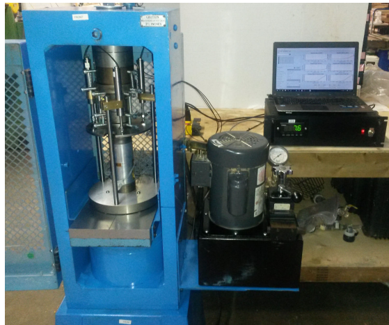
Figure 1: Forney loading frame setup for UCS testing.
