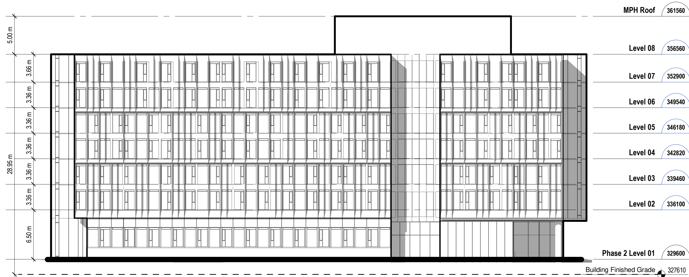
2 Block A - South Elevation AZ401 1 : 250
