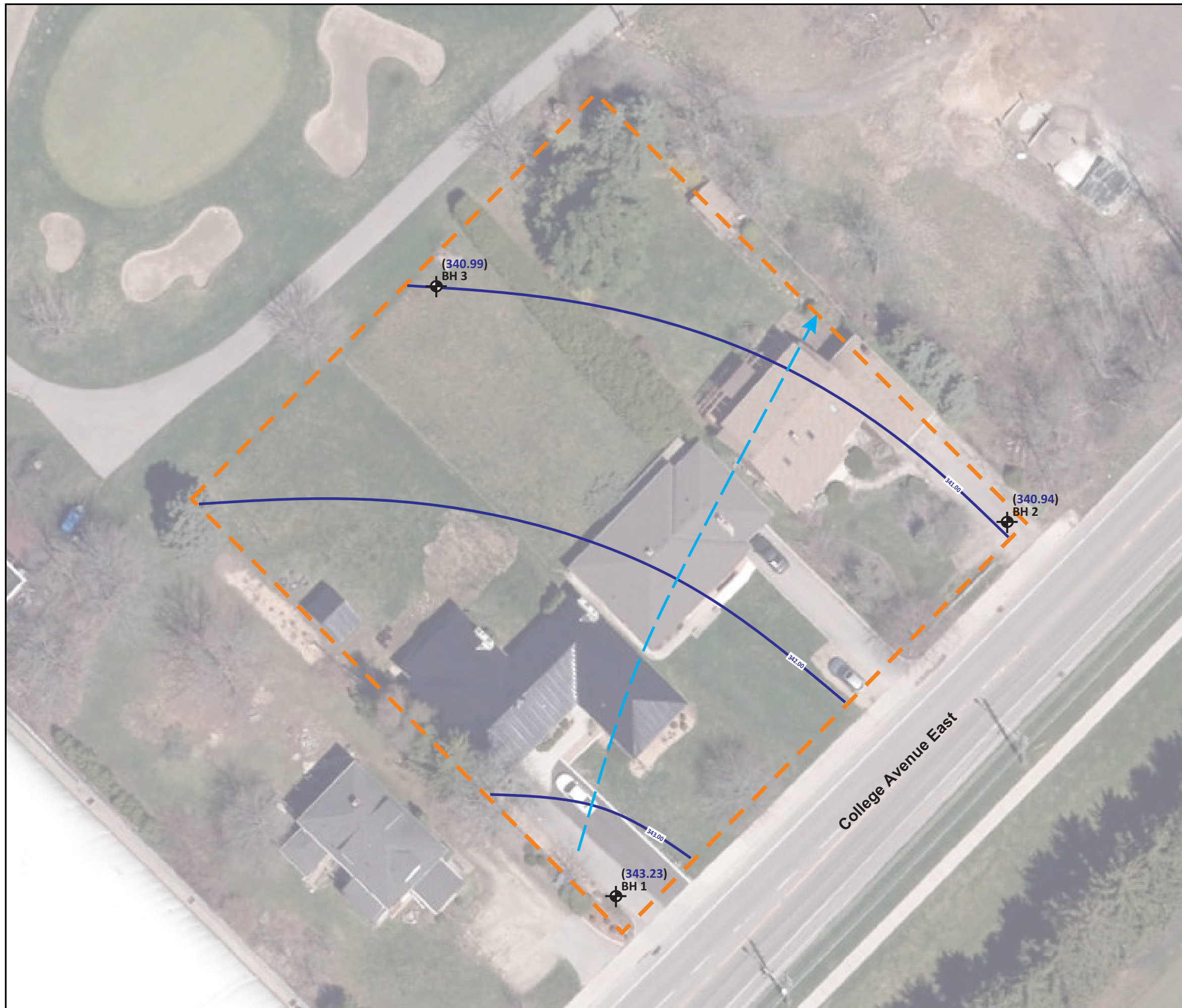
Figure 2: Water Table Interpretation (April 14, 2025) Scoped Hydrogeological Assessment Proposed Residential Development 210 – 222 College Avenue East Guelph, ON
