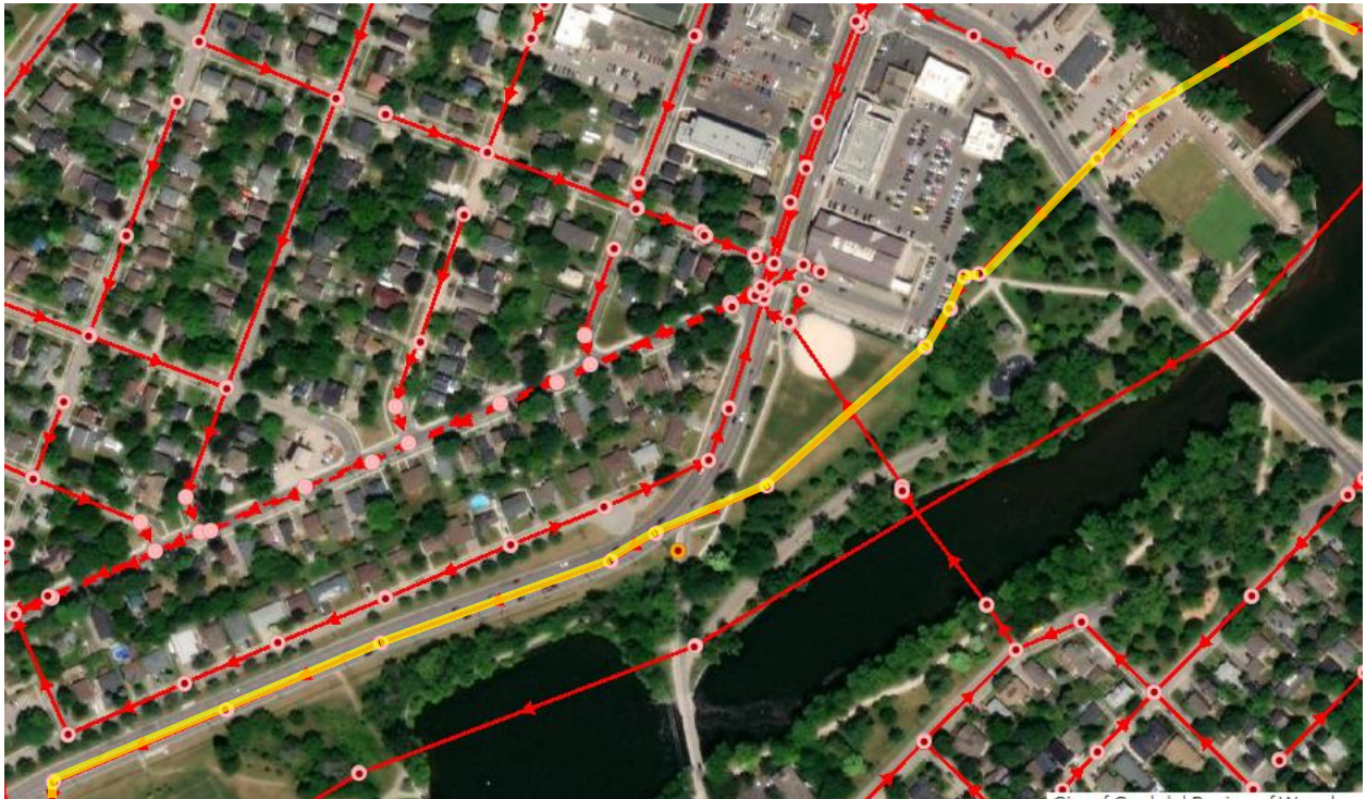
Figure 12 – Aerial View of Surcharged Area 2, Part 3
