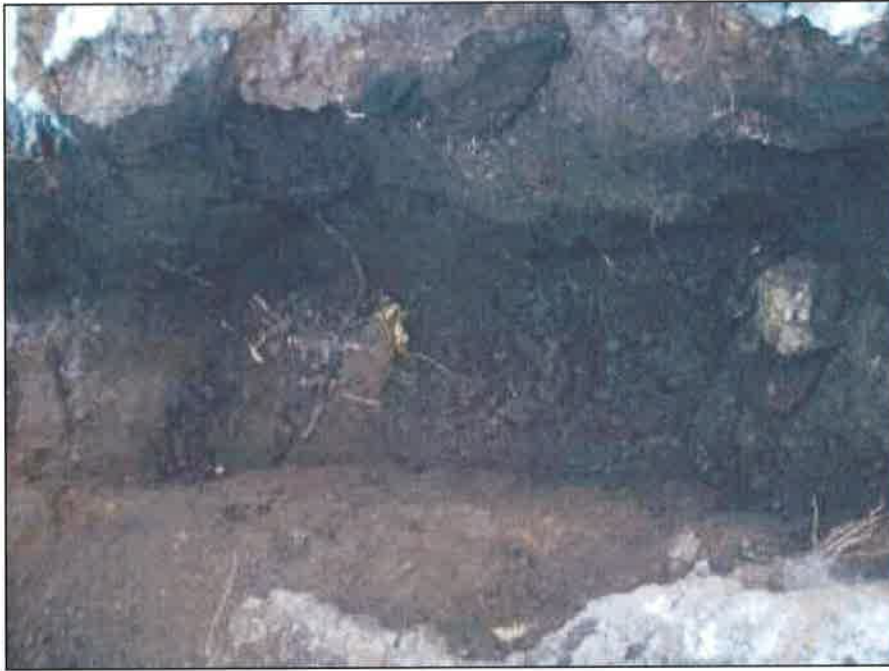
Photo 5 - Mixed topsoil in testhole TH-2. (Later Excavated and removed off-site).
