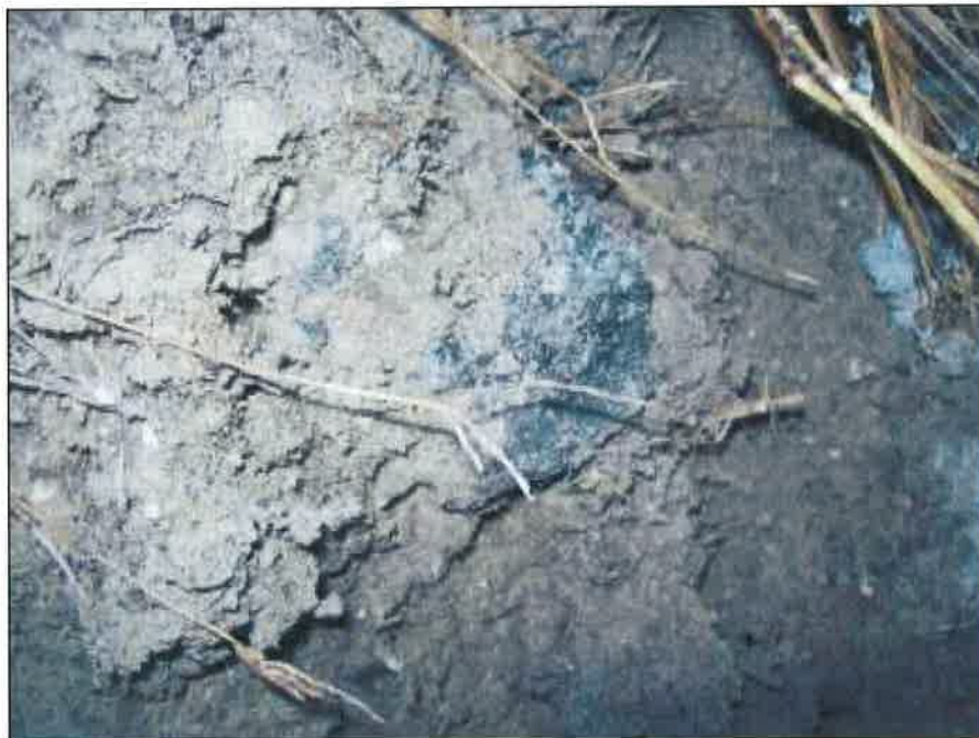
Photo 6 - Mixed topsoil in testhole TH-2. (Later Excavated and removed off-site).
