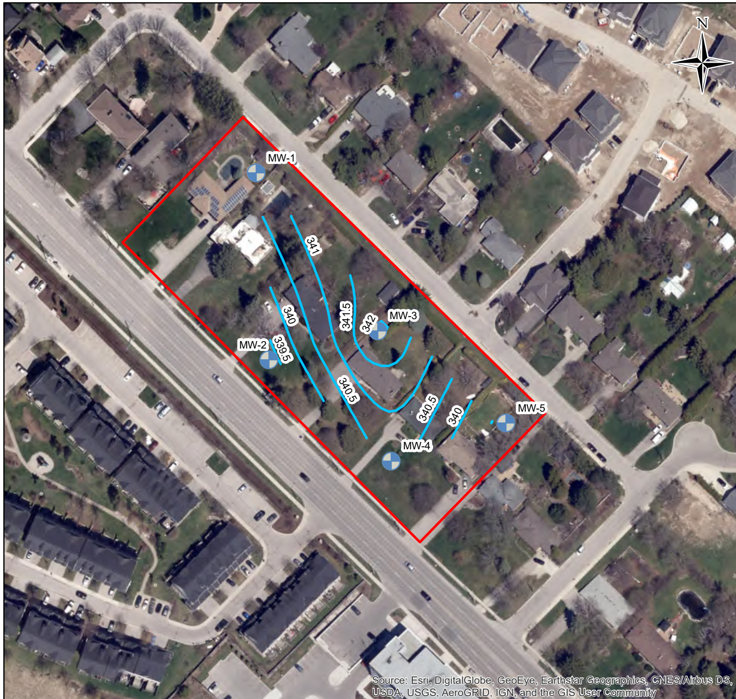
Figure 6: Interpreted Groundwater Contour Plan
