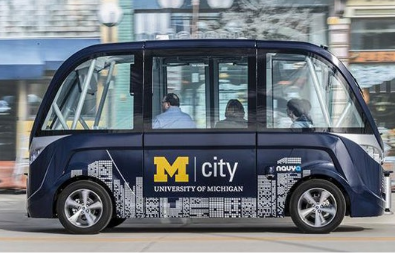
A driverless shuttle at the University of Michigan's Mcity Test facility in Ann Arbor MI. Source: University of Michigan
