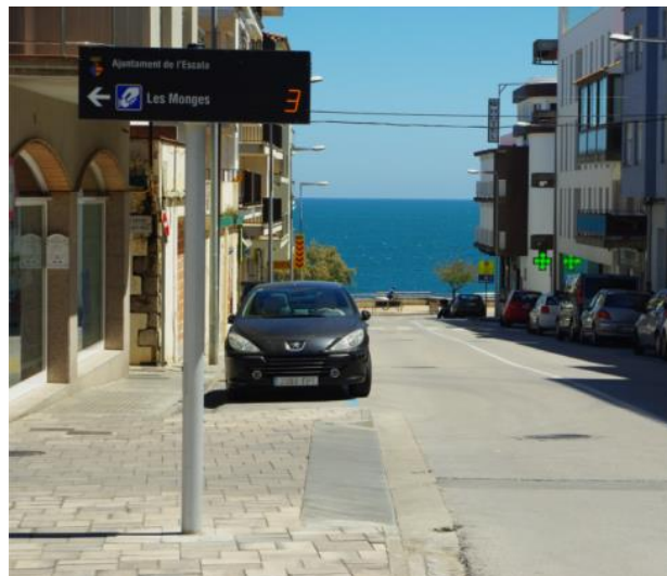
Figure 8: Variable message sign feature of a parking guidance system
