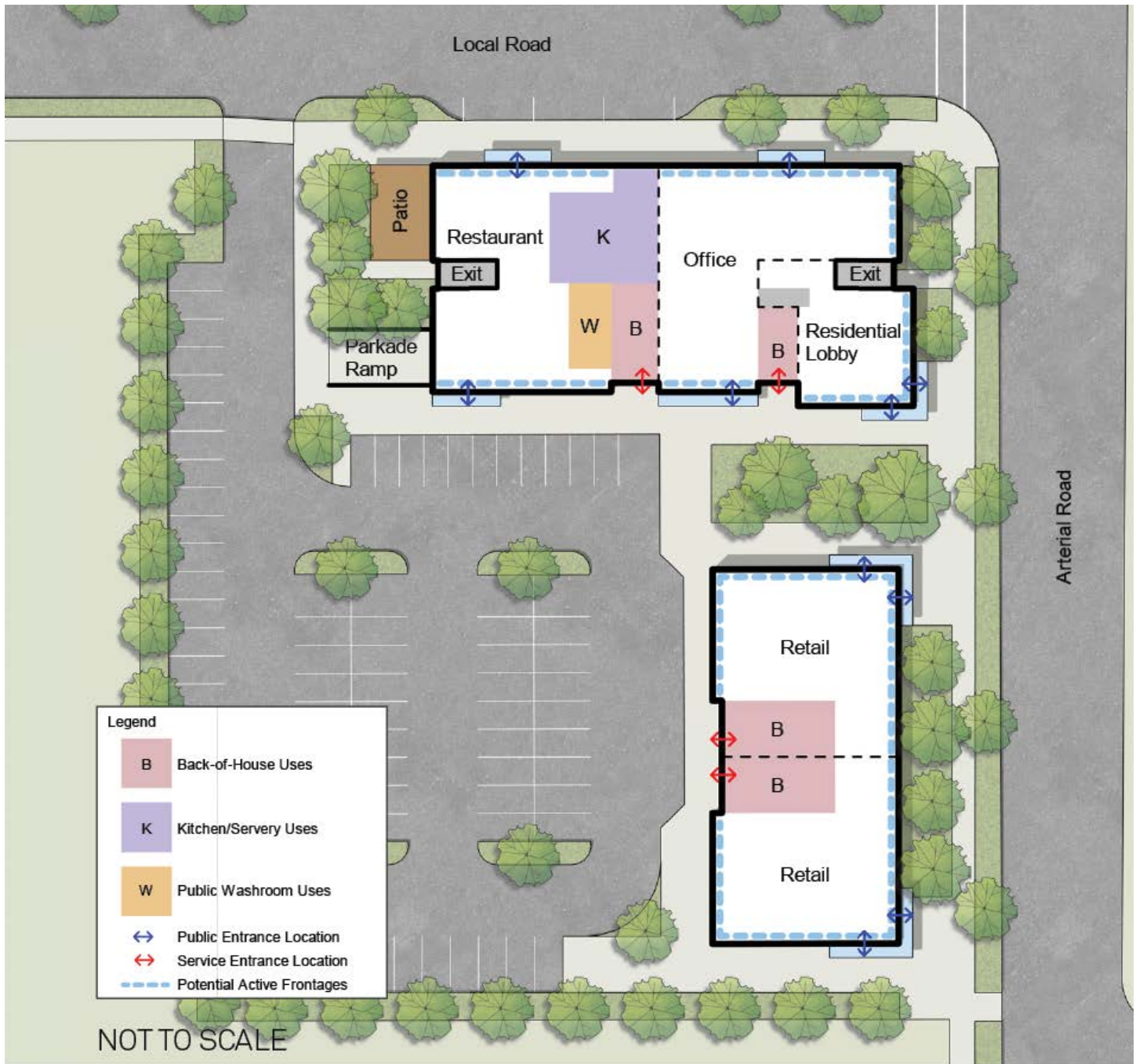
Demonstration plan of commercial site identifying relationship between internal building layout and site and building design
