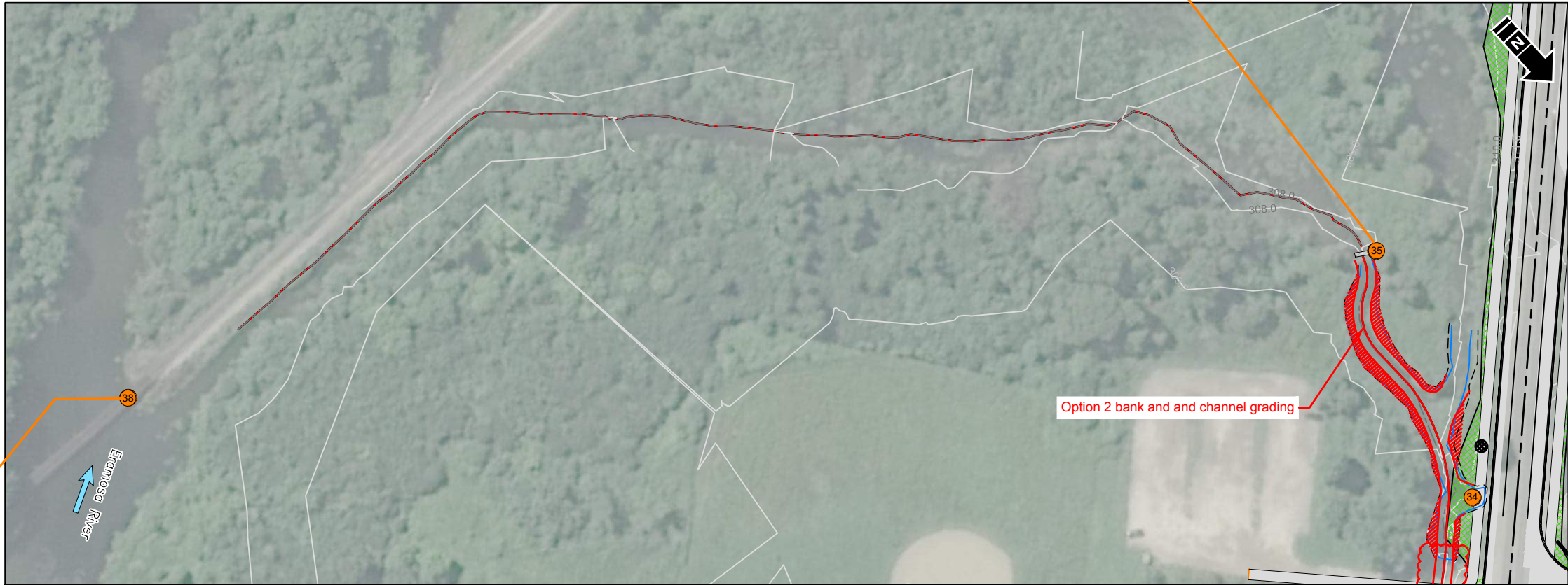
35 Feature #35: Concrete and stone weir (potential significance). Feature to be removed as a result of proposed channel works.
