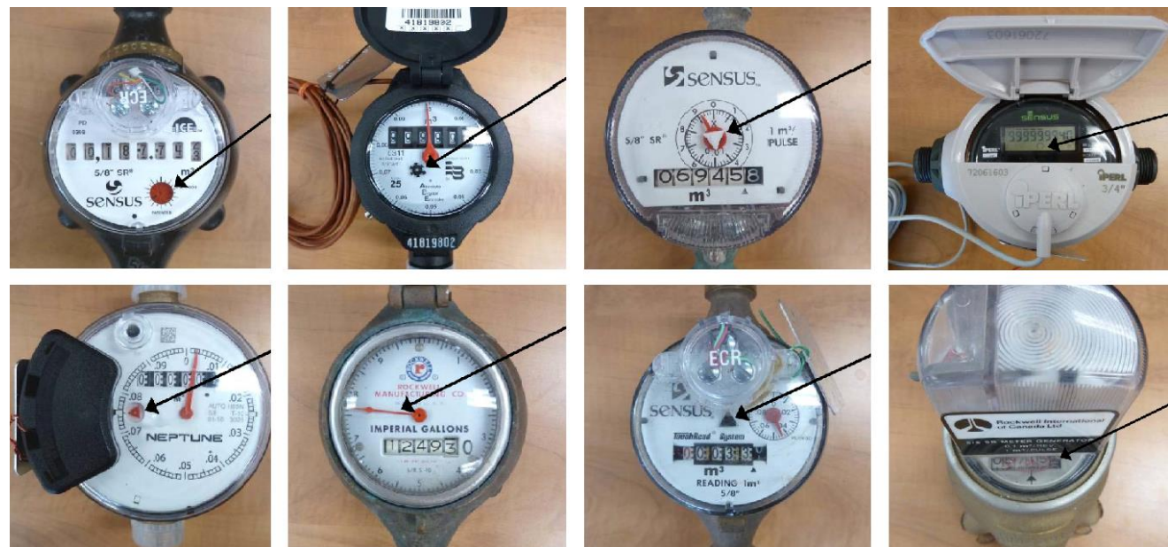
Examples of water meters; arrows point to low flow indicators
