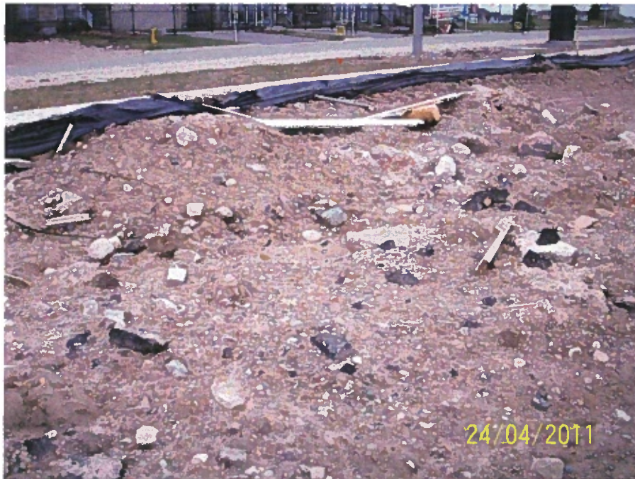
Photo 3: Small area of fill and construction debris along the southern property boundary, which contains concrete, asphalt, wood, plastics and a small quantity of brick.
