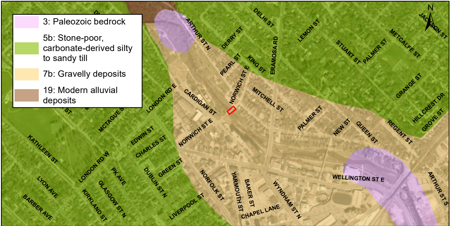
Figure 6: The Ward to Downtown Pedestrian Bridges - Surficial Geology
