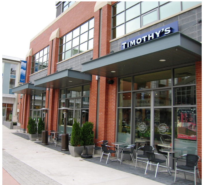
Where active frontage is required, buildings should have a minimum ground floor height of 4.5 metres.
