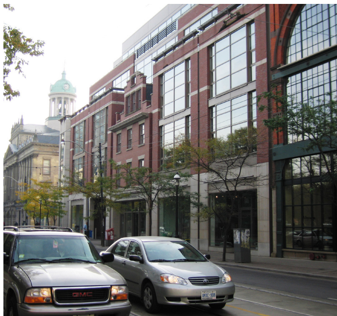
Where frontage exceeds 40 metres, massing should be articulated or broken up to express individual bays.
